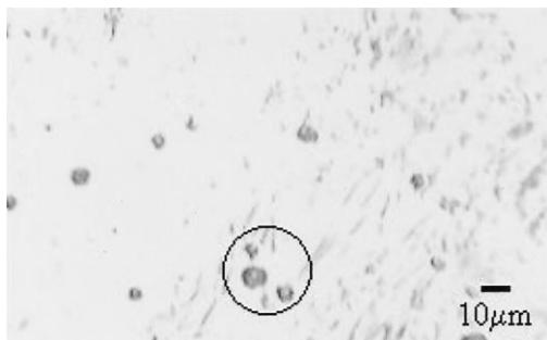
Fig. 8. Photograph of typical macro pores created in Gel I T . The circle diameter is 30 \mu\text{m} . Each macro pore size is quite small compared with those in the other gels.
